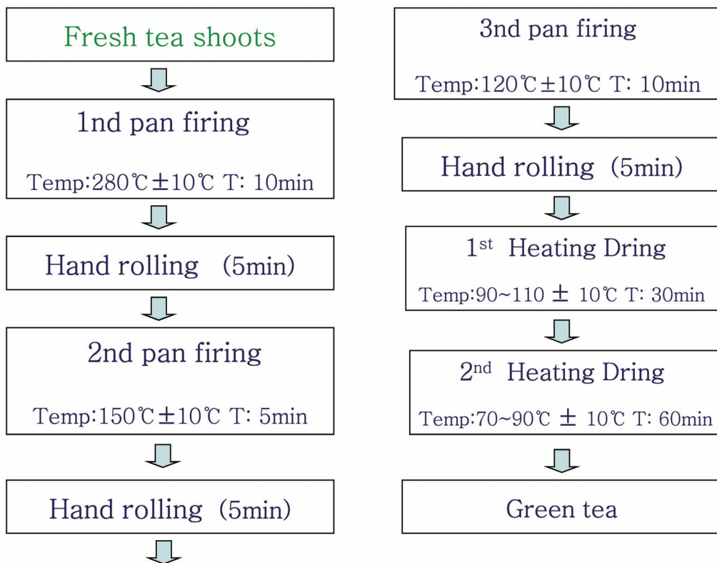
Fig. 1 Green tea manufacture process
