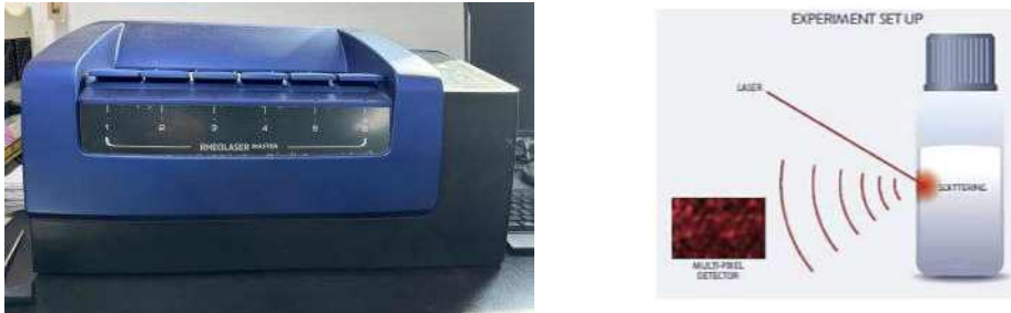
Figure 23. Image and Measuring Mechanism of Rheolaster
