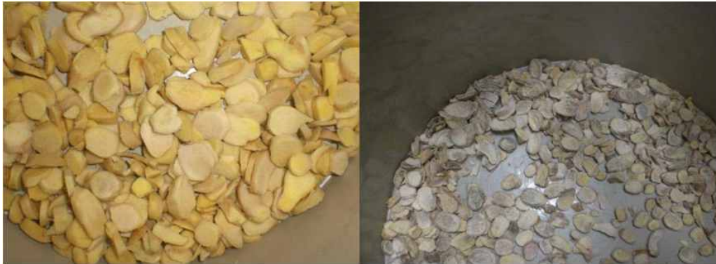
Fig. 13 Morphology of the sliced ginger before (left) and after microwave vacuum drying (right)
