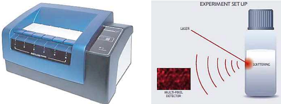
Figure 10. Image and Measuring Mechanism of Rheolaster 71)
