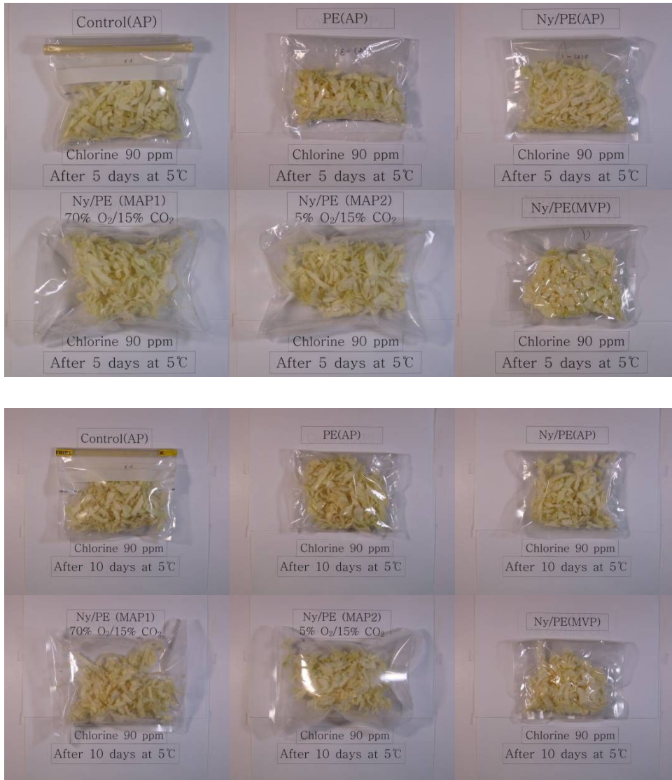
Fig. 51. Appearance of shredded cabbage with hypochlorite solution dipping and various packaging treatments during storage at 5°C. Upper: after 5 days storage, lower: after 10 days storage.
