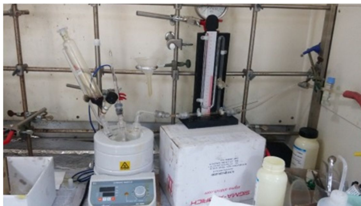
Figure 8. Apparatus for measuring vapor pressure
